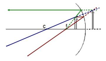
3. Construct the image for an object placed as shown below.
