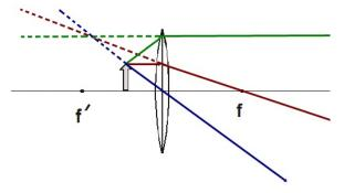
Construct the image formed by the object as shown below. If the focal length of the lens is 15.5 cm and the 3.20 cm (in height) object is placed 22.0 cm from the lens, find (a) the image distance, (b) the magnification, (c) the image height.
